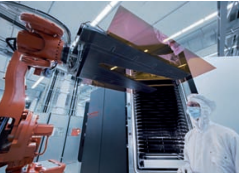
The robot unloads the large glasses of 1.4 m 2 , which have been coated in the KAI 1200 with a silicon absorber layer of less than 0.3 µm.
