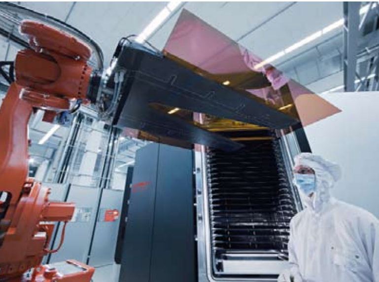
The robot unloads the large glasses of 1.4 m 2 , which have been coated in the KAI 1200 with a silicon absorber layer of less than 0.3 µm.
